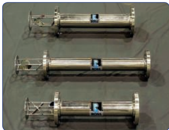
Shown are removable LPD mixing elements supplied with a retainer ring which goes between two mating flanges to keep the mixer from spinning or moving downstream
