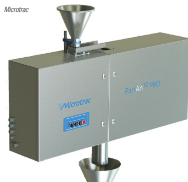
FIGURE 4. The PartAn 3D PRO for process applications uses dynamic-image-analysis technology to measure 36 morphological parameters, including size, shape, surface roughness, sphericity, transparency and 3D in one fast analysis
