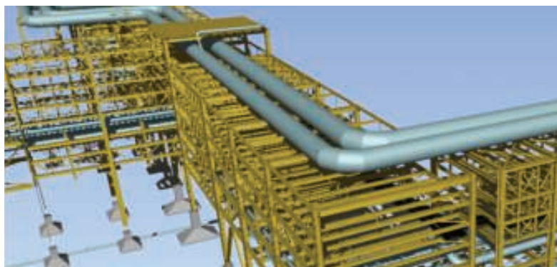
FIGURE 4. This sketch depicts a very high pipe rack to support the main flare header
